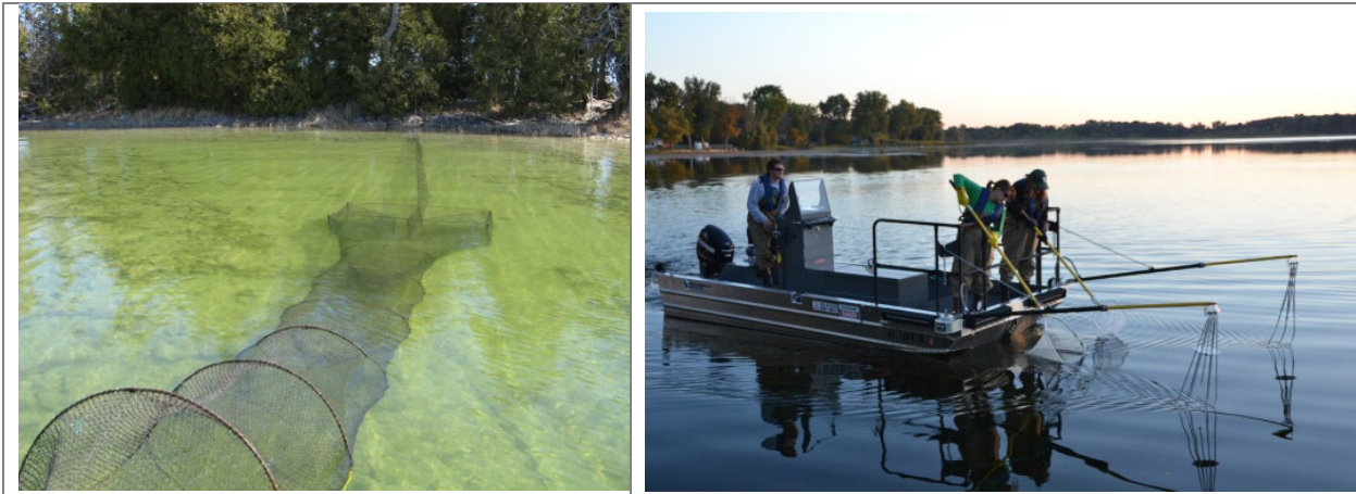
Photograph 3.6-1. Fisheries survey techniques. Fyke net positioned in the littoral zone of a Wisconsin Lake (left) and an electroshocking boat (right).
